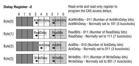
AckWinDelay adjusts the size of the acknowledge window. ReadDelay, WriteDelay, and AckDelay adjust the time from the end of the packet to the start of read data, write data, and the acknowledge packets, respectively.
