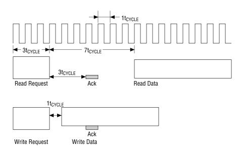
Fig. 8 Sample 16-Byte Read and Write Transactions
