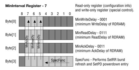
MinWriteDelay, MinReadDelay, and MinAckDelay specify the minimum number of cycles allowed between a request packet and a write data, read data, and acknowledge packet, respectively. SpecFunc is a write-only field that is used to initiate a SetRR burst refresh or to place the RDRAM into powerdown mode.
