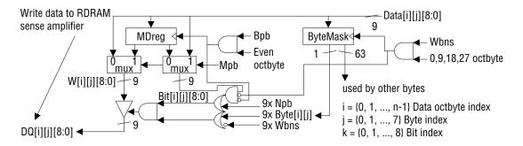
Fig. 14 MDReg with BitMask and ByteMask Logic - one byte slice
