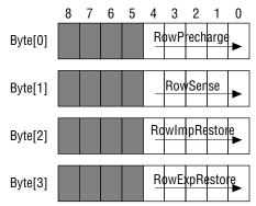
Read-write register to program the RAS access intervals. Note that fields are in bit-reversed order.
