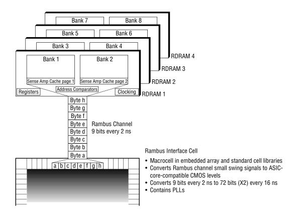
Fig. 3 Data Transfer on the Rambus Channel
