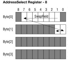
Read-write register for swapping subfields of the Adr field of request packet. This maximizes the row hit rate for many applications. SwapField - Each bit swaps a pair of bits from Adr[28:20] and Adr[19:11]
